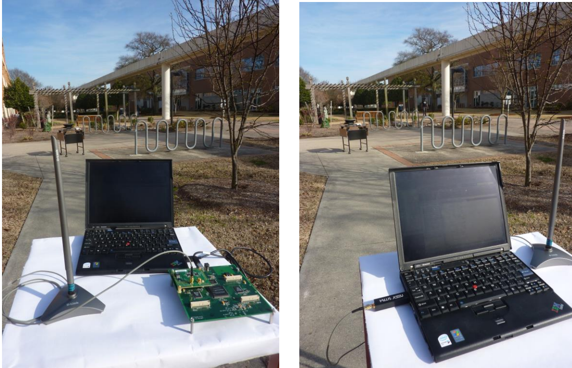
Figure 9. Outdoor transmitter-receiver set-ups for the mobile platform
